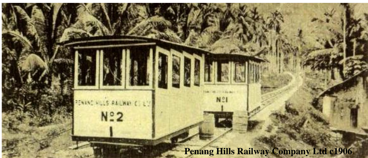
Electrically powered locomotive built from de-commissioned tram parts
